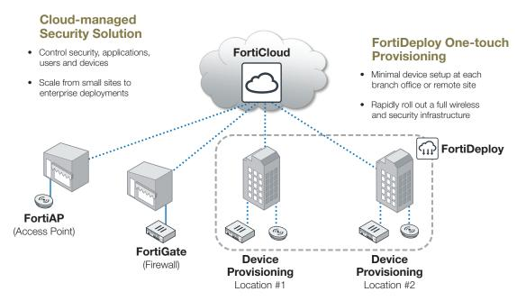
FortiCloud is able to manage FortiAP wireless access points and FortiGate firewalls from a centralized, cloud-based management console.
